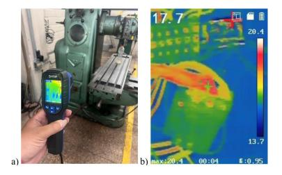
During the operation of the milling machine, higher-than-expected electrical consumption was recorded, as shown in Figure 4. A detailed visual inspection revealed several issues with the electrical conductors, including sections of cables lacking proper insulation and improper splicing, compromising the quality of the connection.
