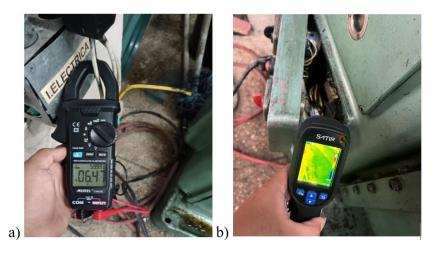
An overcurrent factor of 1.09 was identified in the lathe, indicating a 9% increase in electrical consumption due to faults in its electrical system. This overconsumption signaled a malfunction, causing the lathe to use more energy than necessary. This not only reduced operational efficiency and raised energy costs but also risked accelerated wear of the electrical components.
